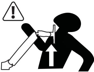
**[EN]** WARNING! Stored Energy Hazard: The arm mechanism is under tension and will move up rapidly, on its own, as soon as attached equipment is removed. For this reason, DO NOT remove equipment unless the arm has been moved to the highest position! Failure to follow this instruction may result in serious personal injury and/or equipment damage!
