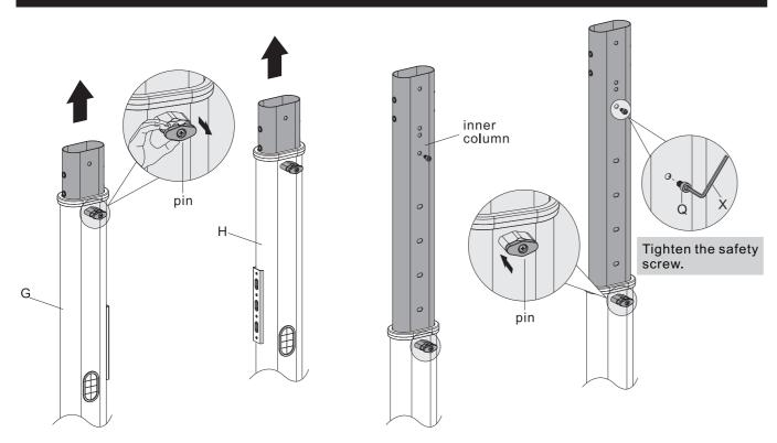
Pull the pin outwards and pull the inner column upwards at the same time, until the inner column is pulled to the desired height then release the pin to secure.
