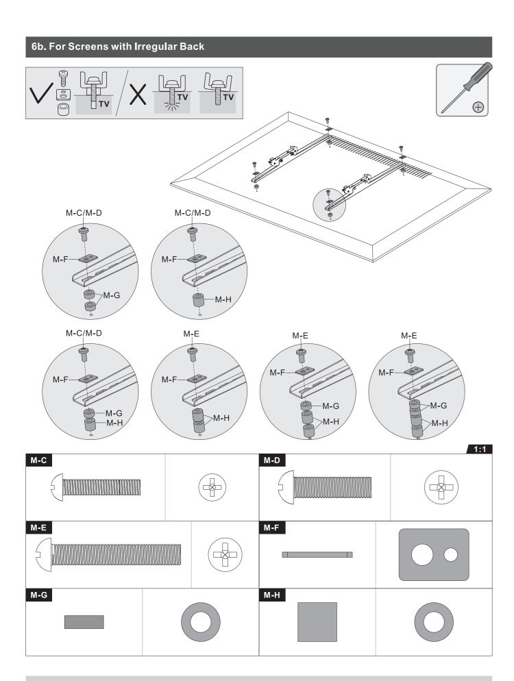
**Note:** Choose the appropriate screws, washers and spacers (if necessary) according to the type of screen. • Position the adapter brackets as close as possible to the center of the display.
