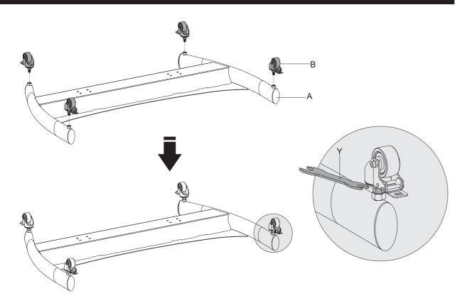
Note: Each caster can be adjusted independently for fine tuning. Slightly turn the nut to lower or raise the base.
