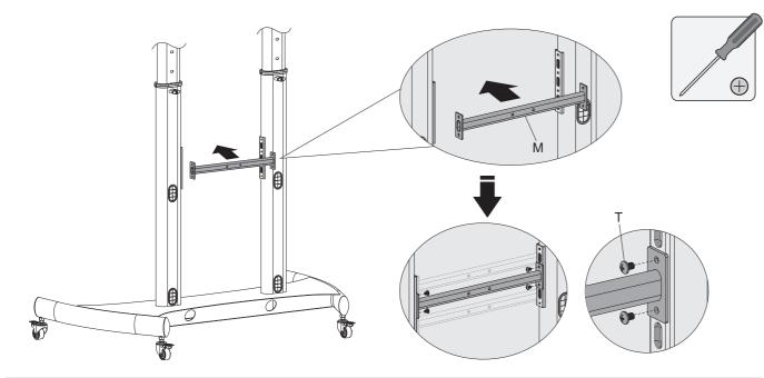
Install the support bar to the columns at the desired position and secure using the appropriate screws.
