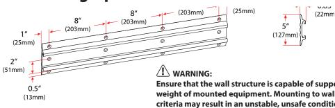
Ensure that the wall structure is capable of supporting four times the total weight of mounted equipment. Mounting to wall surfaces that do not meet this criteria may result in an unstable, unsafe condition which could lead to personal injury and/or property damage. Consult a construction professional if you have any doubt about what this means in regard to your particular application.
